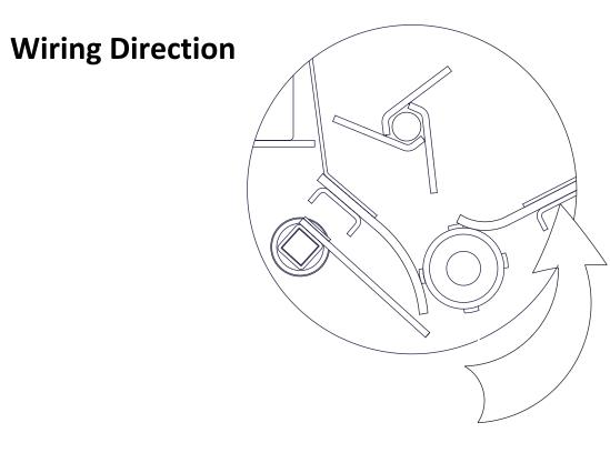
Check direction of distributor drum. To ensure proper rotational direction, wiring may need to be reversed (black-red, red-black).
